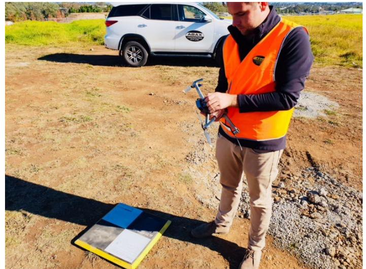
"The AeroPoints are strategically placed around the site and you fly the site with the drone on a preset flight path. Collect the AeroPoints and upload the AeroPoint data and drone images to Trimble Stratus. The dataset is processed and returned within hours, allowing you to analyze and share site maps and models quickly and easily."
